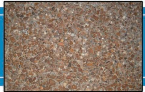
Aggresol-S is a water soluble liquid specially formulated to set the surface mortar of fresh concrete to expose aggregates in freshly placed concrete surfaces. Aggresol-S is green in color to allow for easy identification of applied areas and to ensure appropriate uniform coverage. Aggresol-S should be used to achieve architectural color, texture, and appearance without mechanical means such as sandblasting.
